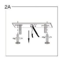
Carefully pull house wires through opening in center of mounting plate. With mounting plate threads facing outward, screw mounting plate into junction box using outlet box screws.
