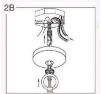
Slip screw collar ring and canopy onto chain, and hang fixture onto screw collar using an open link of chain.
