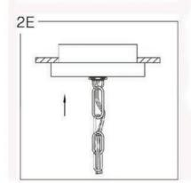
Carefully tuck wires into junction box and secure canopy to ceiling using screw collar ring.
