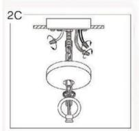
Strip 3/4" of insulation from wire ends. Connect house ground wire to fixture ground wire. Twist wires together using wire nut. Connect the black house wire to the smooth or black fixture wire. Twist wires together using wire nut. Connect the white house wire to the ribbed or white fixture wire. Twist wires together using wire nut.
