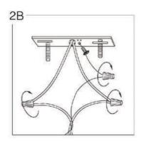
Strip 3/4" of insulation from wire ends. Connect house ground wire to fixture ground wire marked with symbol. Twist wires together using wire nut. Connect black house wire to the fixture. Twist wires together using wire nut. Connect white house wire to the fixture. Twist wires together using wire nut.
