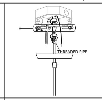
10. Slightly loosen ground screw on mounting bracket (A). Do not completely remove ground screw. Wrap house ground wire (copper) around ground screw, leaving enough ground wire to attach to fixture ground wire. Twist end of fixture ground wire and end of house ground wire (copper) together. Twist wire connector (C) onto ends of wires. Completely tighten wire connector (C). Reference chart below for correct wire connections.
