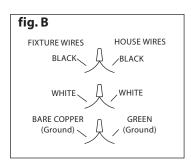
\*Note: To install a post-mount lantern, follow the wiring instructions in section B. When the wires are connected and the fixture is properly grounded, tuck the wires back into the post and slide the fixture post-collar over the post. Secure the fixture with screws (not included).
