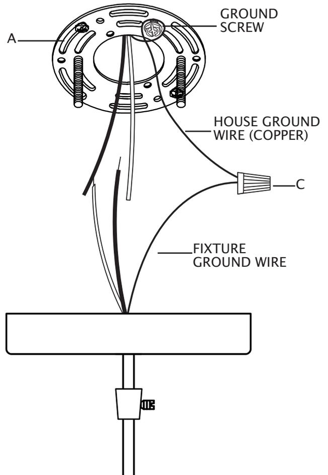
10. Twist end of house lead wire (black) and end of fixture lead wire together. Twist wire nut (C) onto ends of wires. Completely tighten wire nut (C). Twist end of house neutral wire (white) and end of fixture neutral wire together. Twist wire nut (C) onto ends of wires. Completely tighten wire nut (C). Reference chart to the right for correct wire connections.
