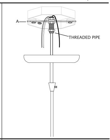
11. Slightly loosen ground screw on mounting bracket (A). Do not completely remove ground screw. Wrap house ground wire (copper) around ground screw, leaving enough ground wire to attach to fixture ground wire. Twist end of fixture ground wire and end of house ground wire (copper) together. Twist wire nut (C) onto ends of wires. Completely tighten wire nut (C). Reference chart below for correct wiring instructions.
