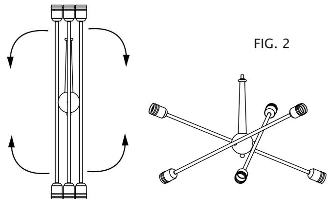
7. Carefully push fixture wires from top of fixture body (O) up through bottom of stem (P). Pull fixture wires out of top of stem (P). Screw bottom of stem (P) onto top of fixture body (O).
