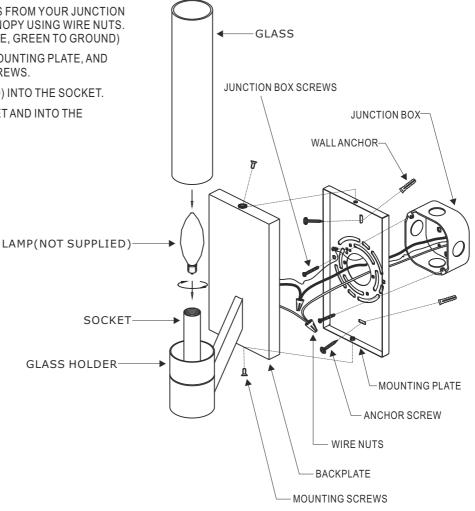
Note: This fixture can only be installed upward.
