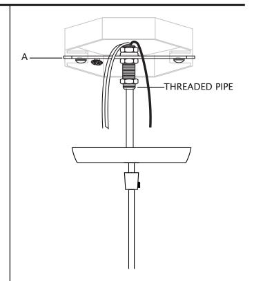
10. Slightly loosen ground screw on mounting bracket (A). Do not completely remove ground screw. Wrap house ground wire (copper) around ground screw, leaving enough ground wire to attach to fixture ground wire. Twist end of fixture ground wire and end of house ground wire (copper) together. Twist wire nut (C) onto ends of wires. Completely tighten wire nut (C). Reference chart below for correct wire connections.
