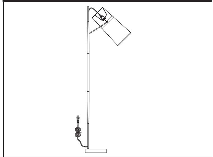
1. From top of base (A), slip long end of threaded pipe (B) through hole in base (A).
